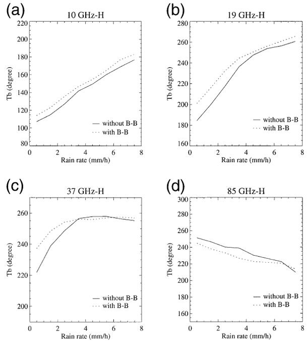
FIG. 1. Mean  $T_{BS}$  (solid lines) and median  $T_{BS}$  (dotted lines) as a function of the PR near-surface rain rates (2A25) for stratiform events with bright band and without bright band for four different TMI frequencies.
