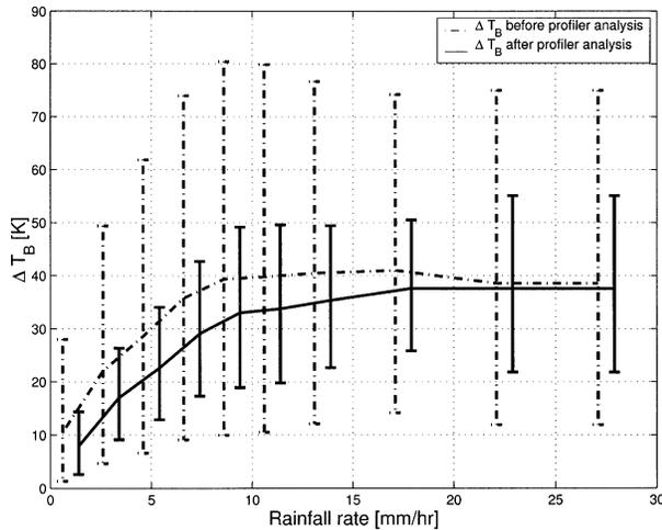
FIG. 7. Mean and std dev of the increase in  $T_{Bs}$  at 10.35 GHz for the cold front case at the CRM resolution as a function of the CRM rain rate at the ground. Note the reduction in the uncertainties in  $T_B$  after the profiler analysis.
