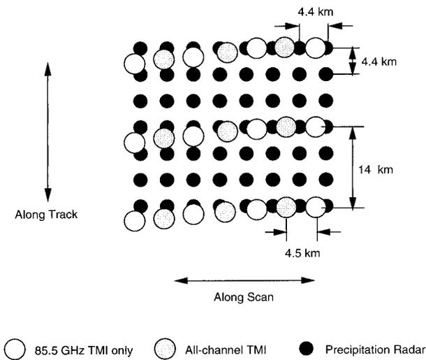
FIG. 11. Scan geometry of TMI and PR.
