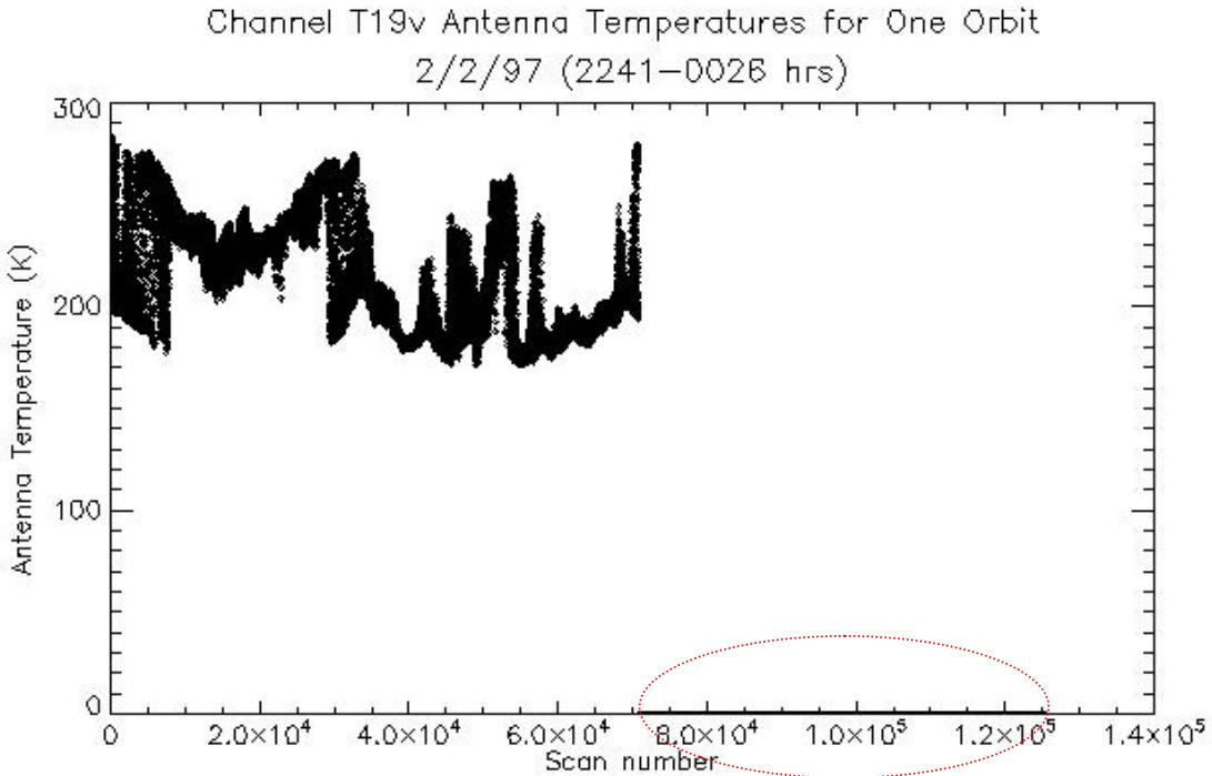
Antenna temperature values toward the end of the scans were assigned zero values. Again, this trend is found across all platforms before 2/4/97. The way this problem was solved was by ignoring the actual number of scans that an orbit claims it holds (number of scans is calculated using either file size or by grabbing the defined number inside the
