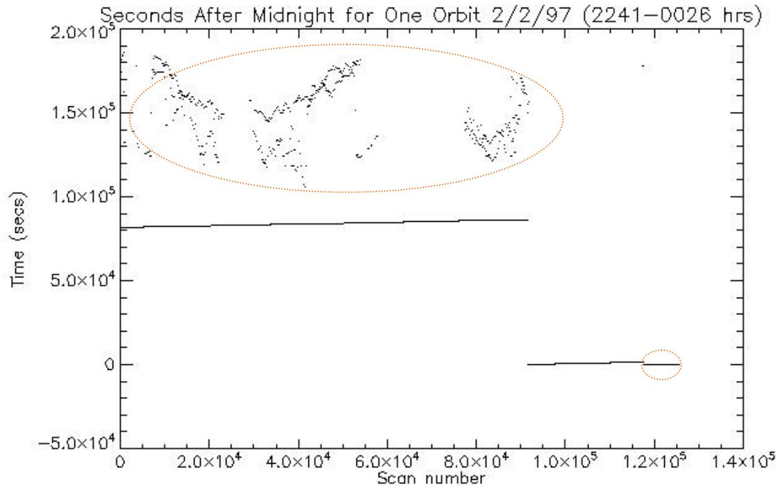
The upper portion of graph shows that time values exceed 86400 seconds ( $>100,000$ ) or time values were assigned zero values as is circled on the bottom right of the graph. The larger red circled area ( $> 100,000$  secs) was eventually eliminated and will be explained later in the report. This same trend can be found for data from all the platforms (F10, F11, F13) before 2/4/97.
