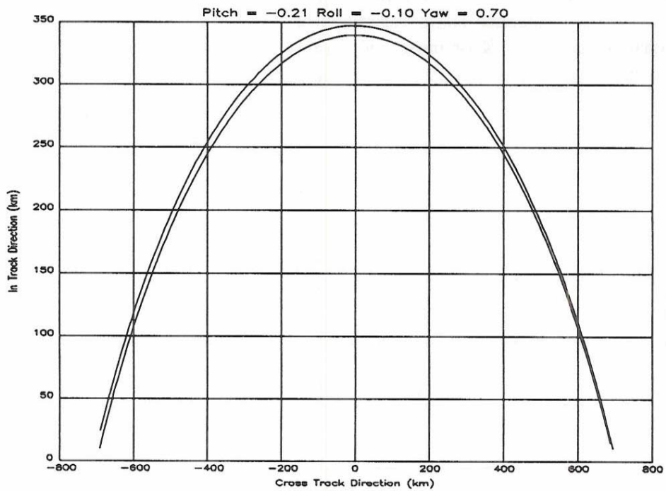
Figure A.14 SSM/I Geolocation Shift Due to Spin Axis Realignment
